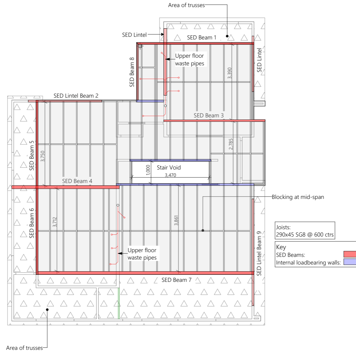
1 Mid-Floor Framing Plan 1:100
